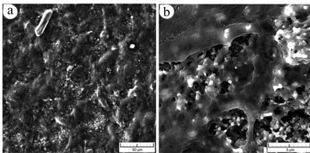
**Fig. 4.** Morphology of TiO<sub>2</sub> coating obtained at induction treatment temperature 800°C after *in vitro* tests for 14 (a) and 28 (b) days.
