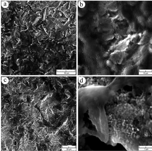
**Fig. 3.** Morphology of titanium (a, b) and TiO<sub>2</sub> coating obtained at induction treatment temperature 800°C and treatment time 120 sec (c, d) after *in vitro* tests for 14 days.
