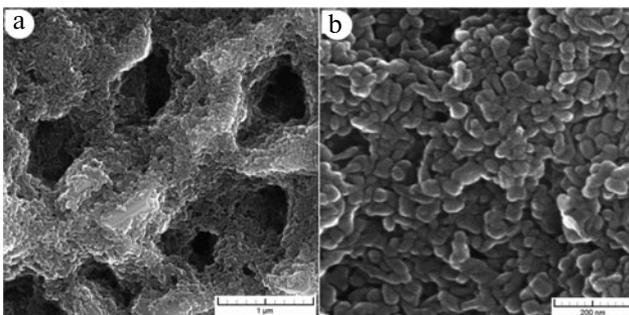
Fig. 2. Morphology of (a) microstructure and (b) nanostructure of coatings obtained at induction treatment temperature 800°C and treatment time 120 sec.
