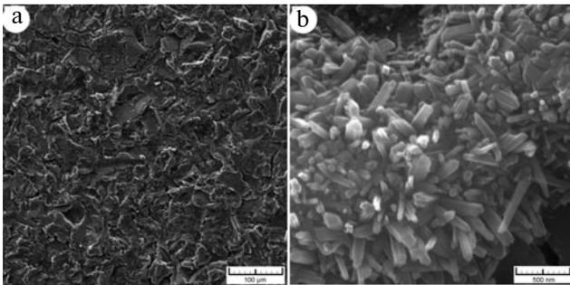
Fig. 1. Morphology of TiO<sub>2</sub> coating obtained in induction treatment mode 600-30: a) microstructure; b) nanostructure.
