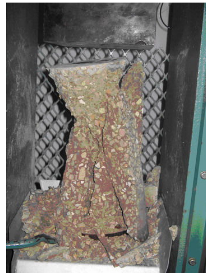
Fig. 1: Failure shape of cylindrical recycled concrete
