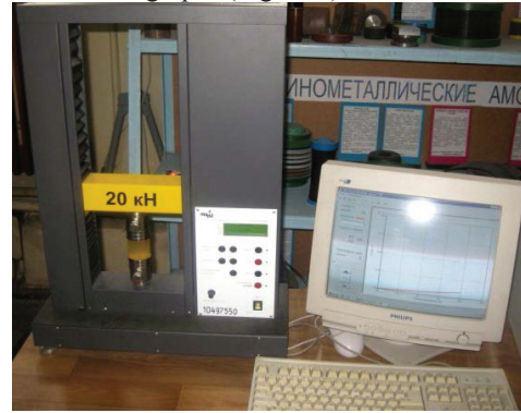
Fig. 2. Small-size desk-type testing machine
