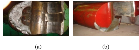
Fig. 1: Destroyed parts of sheet mill mechanical equipment
